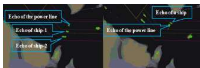
Figure 3: Radar images of power lines and ships across the section of Luotou channel
