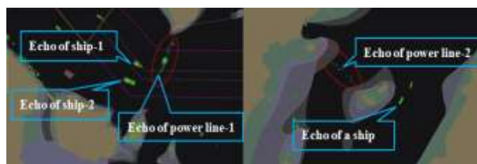
Figure 2: Radar images of the crossing section of Luotou waterway (power line 1) and the crossing section of Qinglongmen-Shuangyumen waterway (power line 2)
