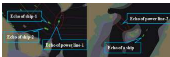
Figure 4: Radar images of ships AIS signals superimposed with the transmission line across the section of Luotou channel
