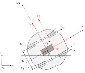
Fig 3: The Motion Model of The Robot
