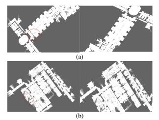
Fig 6: Map built with (a)b1-2014-10-07-12-34-51 and (b)b2-2016-03-15-14-23-01 using Cartographer and the proposed method.
