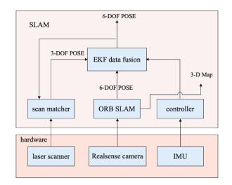
Fig 4: The Frame of the Proposed Method
