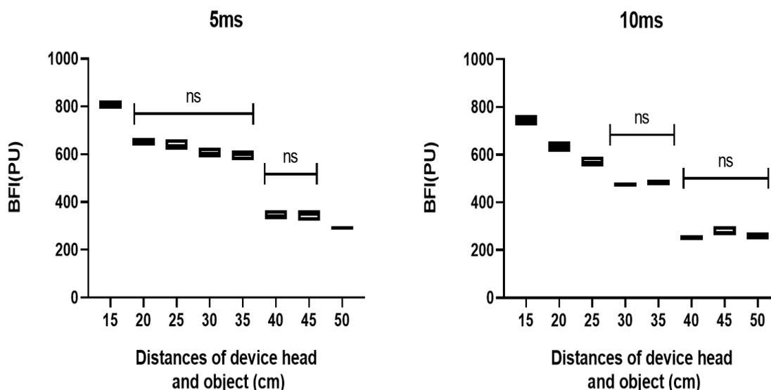
Fig 4: BFI of different distances between the probe and the object under two exposure times.
