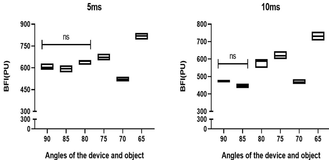
Fig 5: BFI of different angles between the probe laser beam and the object under two exposure times.
