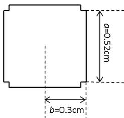
Fig 7: Shape of cross control rod
