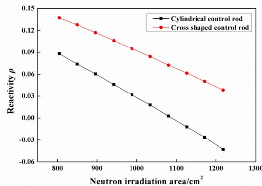
Fig 4: Effect of control rod neutron irradiation area on reactivity
