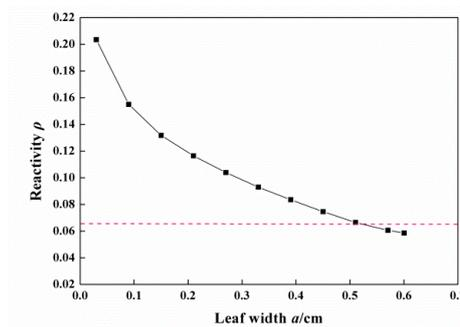
Fig 6: Relationship between reactivity and geometric parameters of cross shaped control rods
