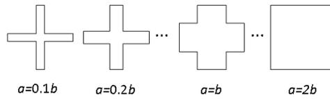
Fig 5: Geometric change of cruciform control rod
