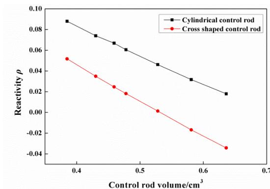
Fig 3: Effect of control rod volume on reactivity
