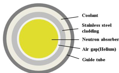
Fig 2: Cylindrical control rod structure
