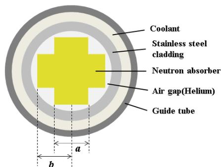
Fig 2: Cross shaped control rod structure
