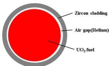
Fig 1: Fuel rod structure
