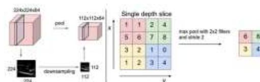
Fig.2 Schematic Diagram of Pooling Operation
