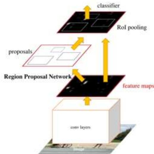
Fig.1 Schematic Diagram of Detection Process of Faster-r Cnn Target Recognition Network
