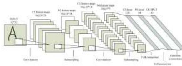
Fig.3 The Network Structure Diagram of Lenet-5
