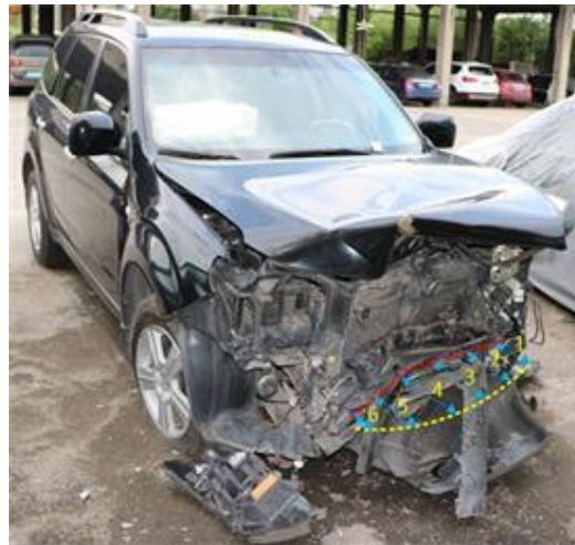
Fig.7 Front bumper measurement method
