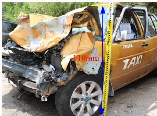
a) On-site measurement of deformation size b) Finite element simulation deformation size
