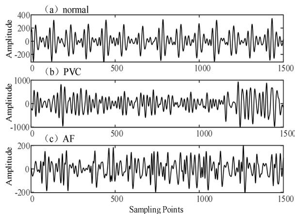
*Fig.2: Example of BCG signals (a) normal (b) premature ventricular contraction (c) atrial fibrillation*
