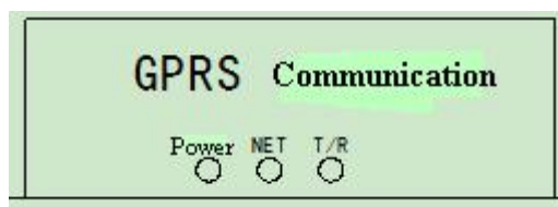
Fig.6 Concentrator Type I Telecommunication Unit Indicator (Refer to Real Object)
